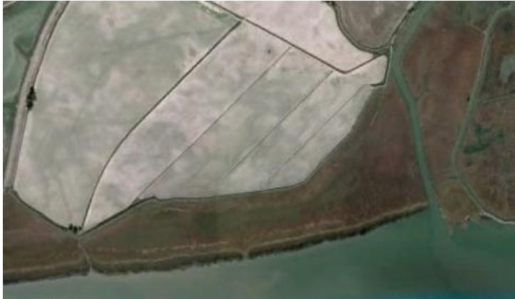
Figure 4. The northern shoreline of San Pablo Bay in the vicinity of Toley Creek, where agricultural fields (former tidal marsh) lay behind levees and fringing marsh that grew on accreted sediments from hydraulic gold mining. Accretion has shrunk the mouth of Toley Creek from a formerly broad channel to a narrow slough.
